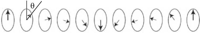
Fig. 5.13. Helical order: Each layer exhibits a ferromagnetic arrangement but the magnetization between adjacent layers is rotated by the angle \theta
